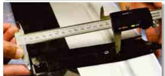
Now the holes for the flaperon connector in the fuselage have been drilled. Protect the fuselage at the appropriate place with Tesa paper tape and draw the centers of the holes. They have to be 133,7 mm from the wall where the trailing edge of the wing leans on the fuselage and 9 mm left and right from the center.
