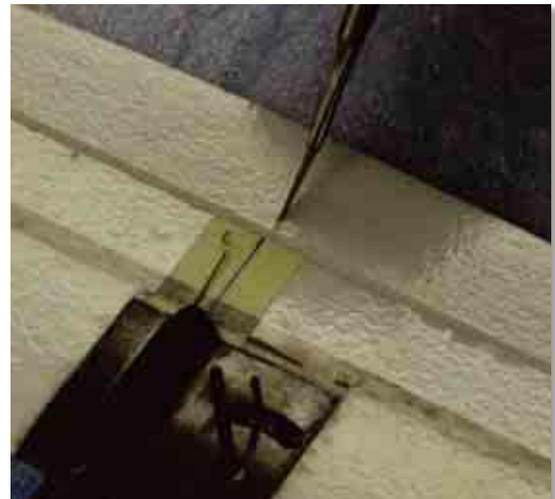
Connect the steel wire for the servo connection to the rudder horn. Insert the rudder horn into the cut. It has to be rectangular to the surface and it is VERY important that the hole on the rudder horn is exactly above the hinge.
