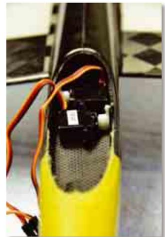
Now the servos for the horizontal and vertical tail have to be installed. Note that we have installed the servo for the horizontal tail nearer to the flaperon servos but you can install the servo for the vertical tail first. Also be careful that you will be later able to install the battery and the receiver.
