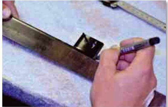
Now we have to get the exact measurements for the mounting point of the vertical tail (rudder box) that is molded to the fuselage. The depth we measure as near to the fuselage as possible. It should be somewhere near 40 mm.
