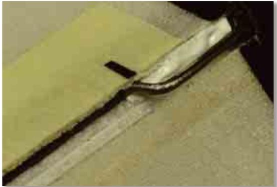
Push the connection the whole way into the hole and cover it with micro-balloons.
