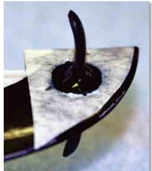
Apply mixture of 24 hour epoxy and micro-balloons into the hole that was drilled in the flaperon for the flaperon connection.
