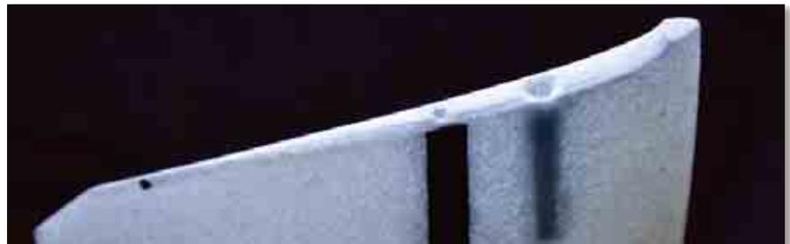
It can be necessary to sand away a bit of the fuselage as shown on the picture to achieve a really tight fit.
