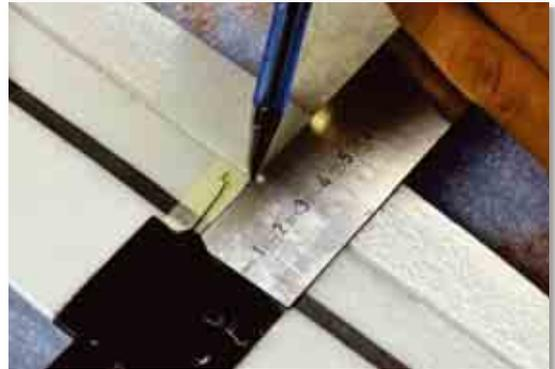
Once you have defined the place make as small cut in the rudder with a scalpel or sharp knife. The cut has to go down to the second layer of glass fiber on the other side but not thru it.
