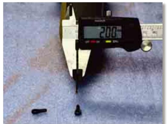
Now we suggest making some notches into the  $\varnothing 2$  mm carbon rods on one side as shown on the picture
