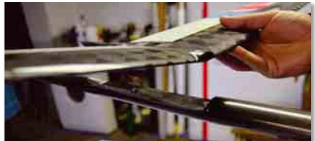
Be careful that the nuts are not turned around when screwing on the wing. But you should nevertheless screw it tightly on.
