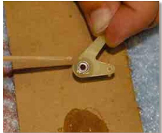
Before the glue hardens assemble one half of the tail with the carbon rods and the bell crank as shown in the picture. This will ensure that the bearing is positioned in the correct position. Leave the glue a while to harden.
