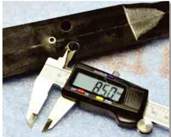
There are two more holes to be drilled on the outer skin of the fuselage for the later mounting of the ball heads.
