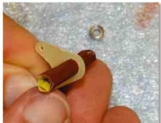
Sand the bell crank around the hole to prepare the surface for gluing.
