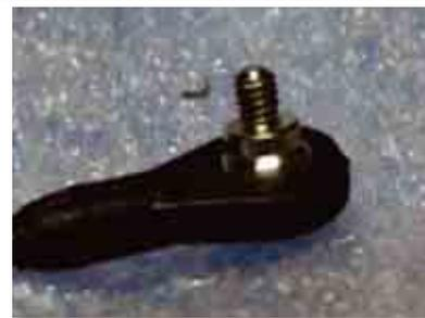
The sanded ball ends have to be mounted on the wing side.
