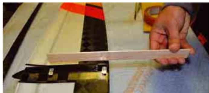
Once you have glued the nuts to the piece of balsa you are ready to glue them into the fuselage.
