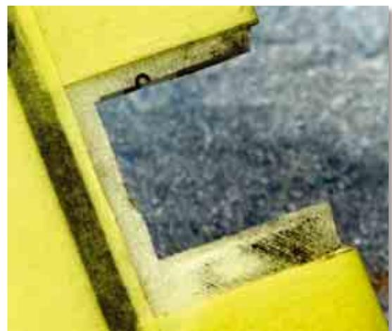
Take the rudder out and sand the marked piece away, so that it will not obscure the movement of the bell crank. You can mark it with a pencil so you will be precise. Place the rudder back on its position and check it.
