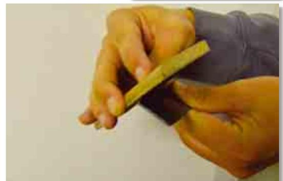
Sand the servo board on both sides. The whole top side, where the servos are mounted, has to be sanded, on the bottom side only 5mm from the edge have to be sanded. (Sand paper granularity 500)
