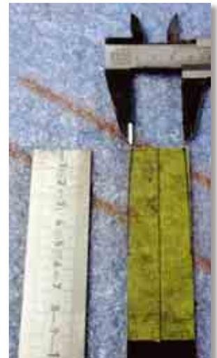
Now the board is in shape, it still has to be sanded in angle so that the glue surface is as large as possible (angle approximately 60°). (Sand paper granularity 120)
