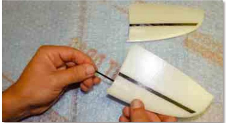
Sand the ends of the 1.5 mm carbon rod just so much that you remove the edge.
