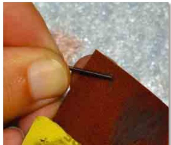
To prepare the bearing for gluing sand it. We use the method shown on the picture but normal sandpaper will do to.
