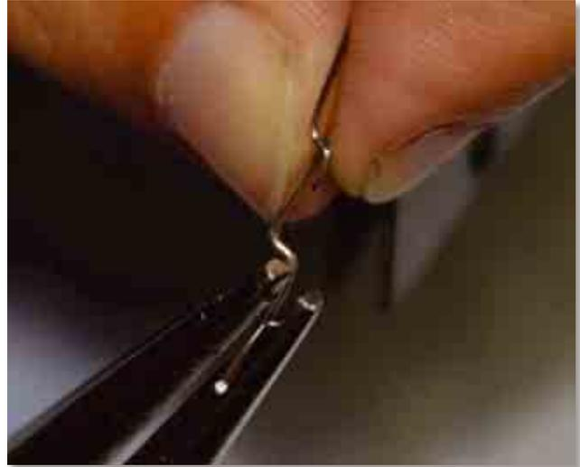
Assemble the bell crank with the pushrod.
