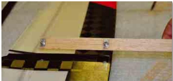
To glue the nuts into the fuselage use **5 min. Epoxy**. A release agent was already applied to the wing and the fuselage on the appropriate places so you do not need to worry about that.
