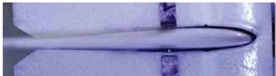
Now the part of the horizontal tail that prevents the rudder to move has to be cut away. For this mount the horizontal tail and mark it exactly at the hinge.
