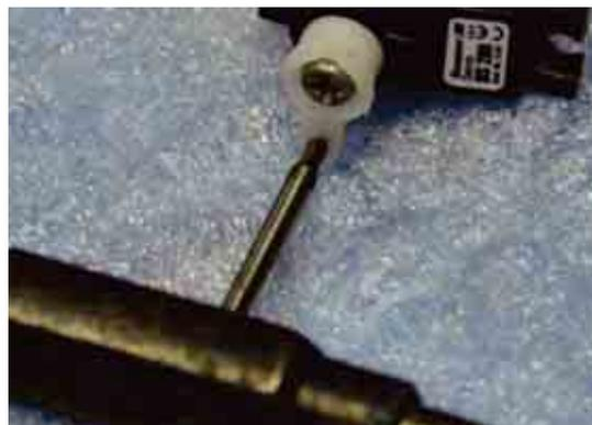
If you have looked carefully you have noted that the four large ball ends supplied are different. Two have been sanded so that there have more space to move in the housings, two are standard ones. The standard ones are mounted on the servos.
