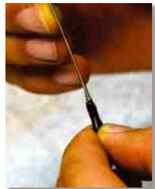
Once the glue hardens apply some super glue on the  $\varnothing 2$  mm carbon rod and push the  $\varnothing 3/2$  carbon rod down to the ball end housing.
