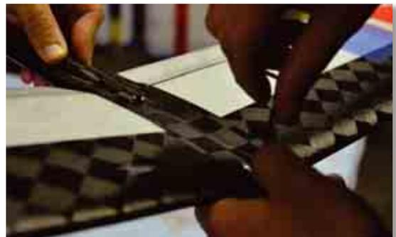
Be careful to adjust the wing precisely to the fuselage. The middle line on the wing and the fuselage is a good point of reference ;-).
