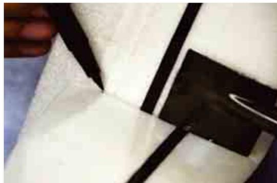
Now cut away the appropriate part of the horizontal tail so that you achieve the rudder movement you desire. We recommend cutting it away parallel to the already prepared line, but if you want you can cut away less (more we do not recommend). Note that the mark made in previous steps was also cut away.
