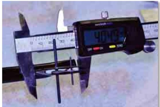
Next we measure the part below the middle point that we determined previously. It should be around 13 mm.
