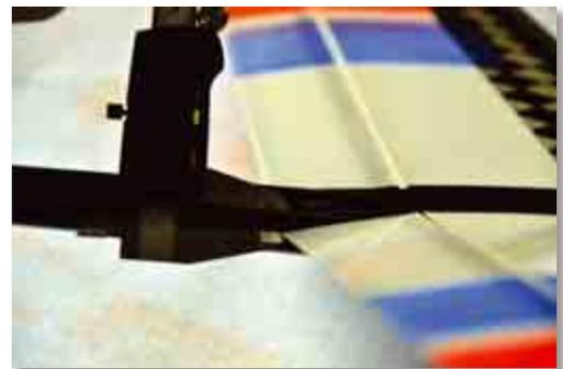
Cut the pushrod onto the appropriate length and make some notches into them as shown on the picture
