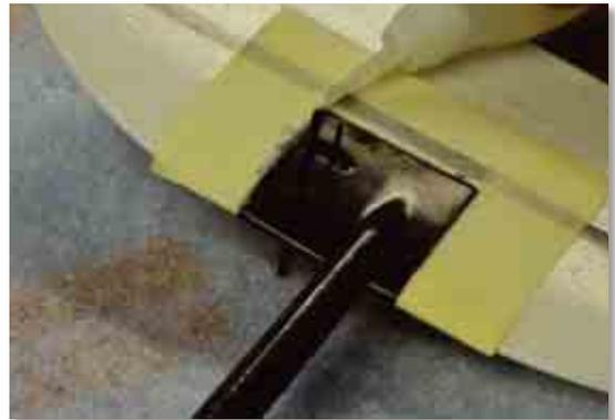
The only thing left to do is to glue in the ruder horn. To do this you have first to determine where it should be placed. This have to be done in the middle of the space prepared in the fuselage. The fuselage has a widening so that the rudder horn can be as long as needed and move freely. Do it as Shown on the picture.
