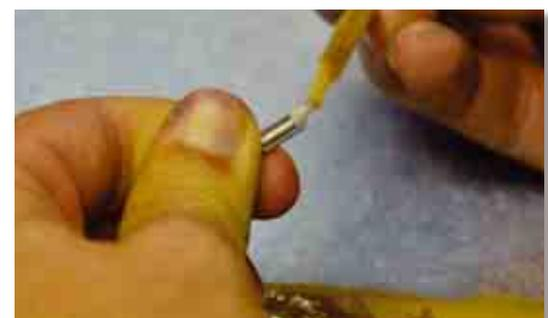
Leave the ball ends screwed on while gluing so that you do not get glue on the thread. If some excess glue was pushed out of the holes wipe it off. Both installed ball heads should have the same distance from the wing. The end result should look like shown in the picture. Once the glue has hardened unscrew the ball ends.
